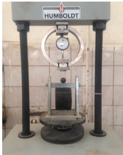
Fig. 4. Indirect tensile tester with a loaded sample.
